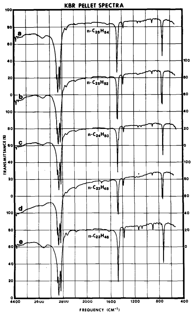
FIG. 9—Absorption spectra of five normal hydrocarbons in KBr pellets: (a) hexacosane, (b) pentacosane, (c) tetracosane, (d) tricosane, and (e) docosane.
